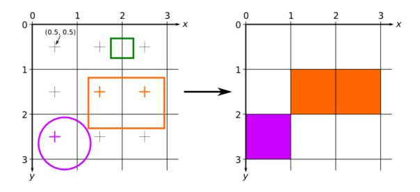
Figure 0.1: Diagram showing a how pixel output is calculated by the GPU given the mathematical description of several shapes.
